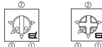
3314J-3, G-3, R-3, H-3 (Reverse Marking, Straight Slot) 3314J-4, G-4, R-4, H-4 (Reverse Marking, Cross Slot)
